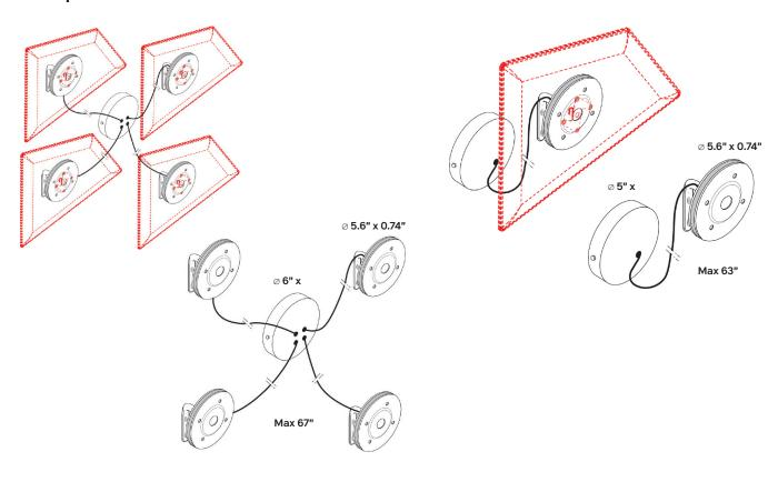
Actual project diagram using FLAT LED Light (finished installation on last page)
