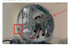
02. Depending on the length needed to run FLAT LED power wires behind the wall, cut wires at the appropriate length (approx. 7" from housing); strip plastic to expose copper wire ends.
