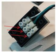
06. Run wires from LED Circular light behind wall and run to corresponding wire that was previously cut. Using included wire connector, connect wires appropriately.
