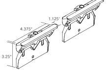
Pair of wall brackets come in either in a satin nickel or matte white finish. (Screws to fasten bracket to wall not included).
