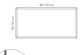
Designed to fit in a 2' x 4' (.61m x 1.22 m) acoustical drop ceiling grid. Fine line grid & T-bar grid compatible.
